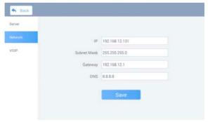
IP: the system will automatically display IP address of the nurse terminal.
