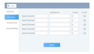
Note: When the bedside terminal calls the nurse terminal, if the call is not answered within the set time, the system will automatically transfer the call to the nurse terminal and so on. The call will be connected level by level.
