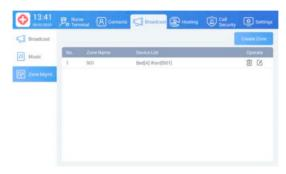
Clicking "Create Zone" icon, the system will enter into the following interface: Enter the zone name, then select and add the device (ward door terminal or bedside terminal). Click the "OK" icon to finish creating the zone.
